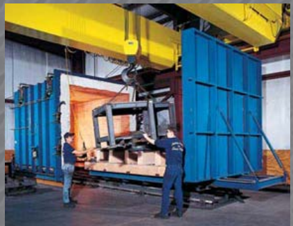
Stress relieving/annealing in PGI's 40,000 lb. capacity furnace.
