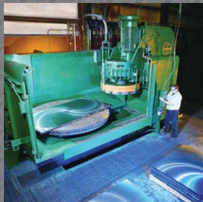
Blanchard grinding with 129-inch swing capacity.
