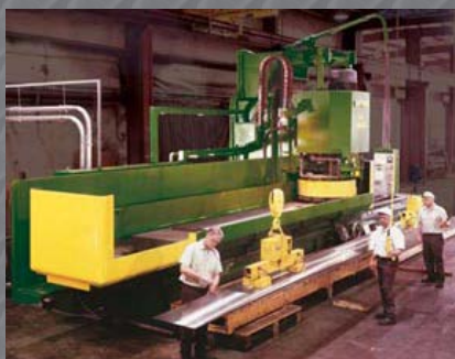
PGI's 415 HP Mattison 400-S vertical spindle surface grinder with 48" x 200" capacity.
