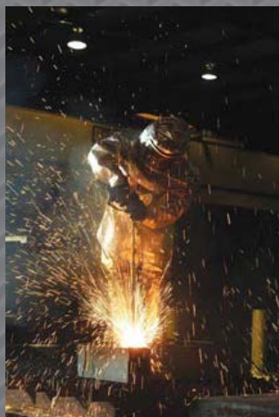
Lansing of thick plate in PGI's plate cutting department.
